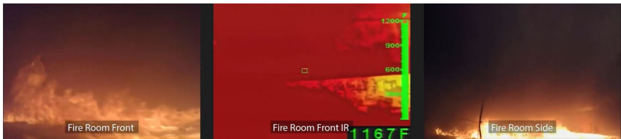
Figure 5.26: Experiment 6 - Conditions in the fire room at 420 s after ignition.
