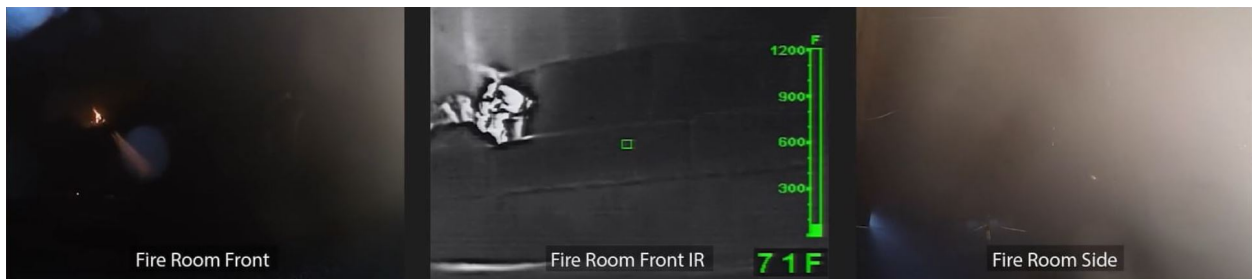
Figure 5.20: Experiment 4 - Conditions in the fire room at 736 s, 10 minutes after nozzle activation.
