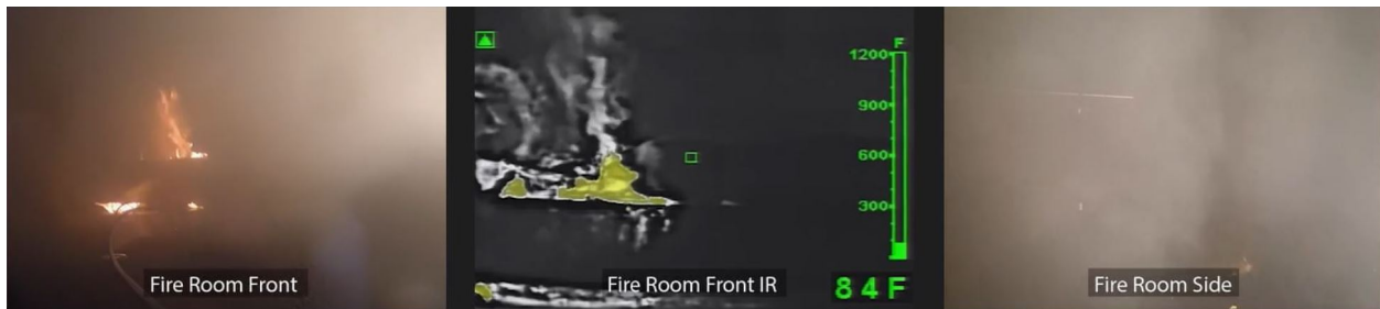
Figure 5.4: Experiment 1 - Conditions in the fire room at 750 s, or 10 minutes after sprinkler activation.
