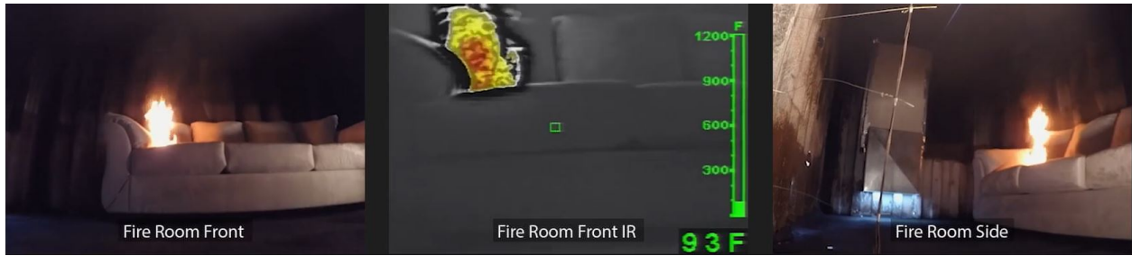
Figure 5.23: Experiment 6 - Conditions in the fire room at 120 s after ignition.
