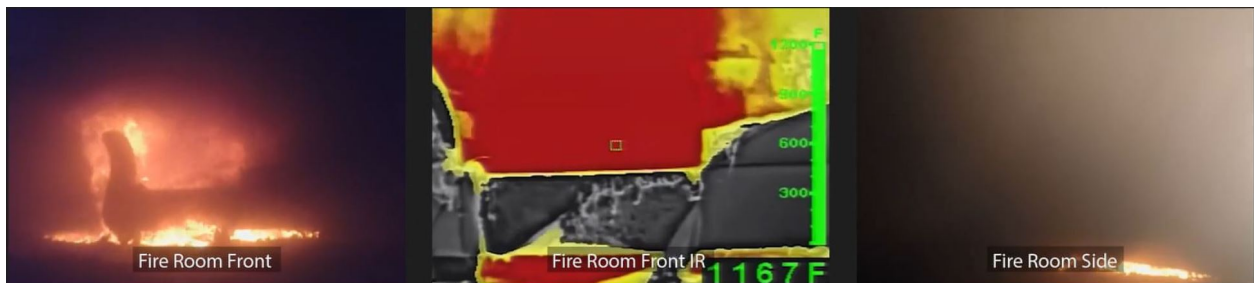
Figure 5.25: Experiment 6 - Conditions in the fire room at 300 s after ignition.
